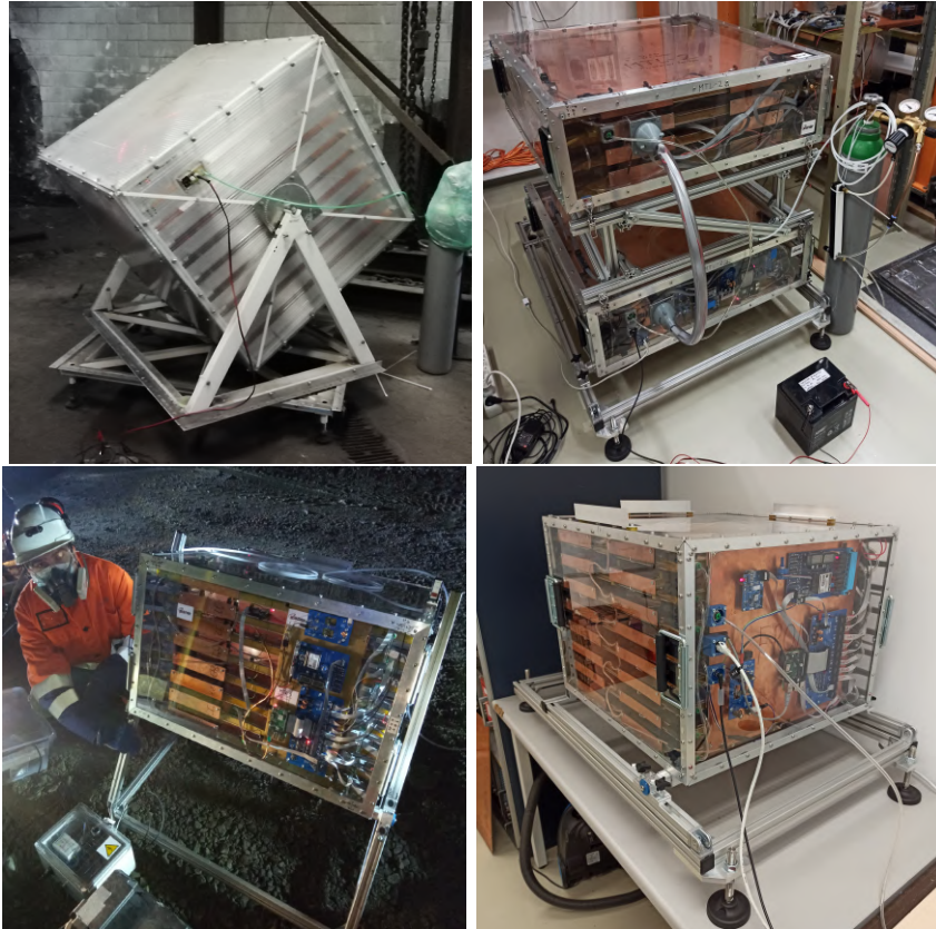
Figure 3.13: Photos of the underground MWPC modules: 'MTL-1' in top-left (muograph with type 80 chambers, on its inclinable rotatable support), 'MTL-2' in top-right (80 cm muograph with two detachable parts), 'MTL-3' in bottom-left (an 80 cm muograph deployed in the Kemi mine, Finland), and 'MTS-50' in bottom-right (compact type 50 muograph).
