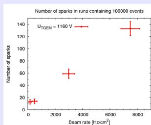
For a give gain the sparking probability is linear with the beam rate till 8000Hz/cm<sup>2</sup> (our measurable limit).
