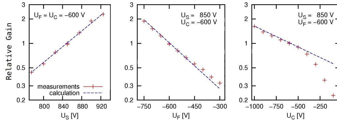
Gain vs sense wire voltage was measured as the only input parameter for the simulation (gain depends on the gaseous filling as well).
