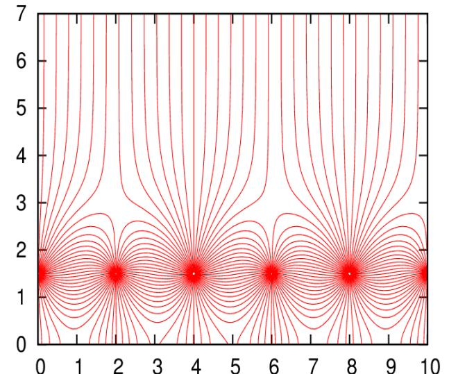
There exists a certain voltage configuration where sense wire charge and therefore gain does not depend on the padplane distance
